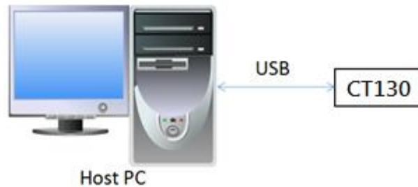
Figure 10-1 connect CT130 board to Host PC via USB port
